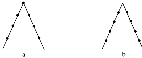
FIG. 2. Examples of the placement of gridpoints near a corner.
